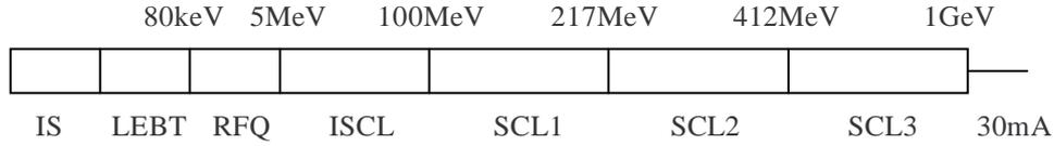
Figure 1: The block diagram of the ADS accelerator
