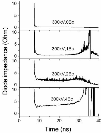
Figure 5: The diode impedance histories at various externally magnetic fields.
