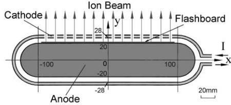
Figure 1: Schematic of a planar MID.
