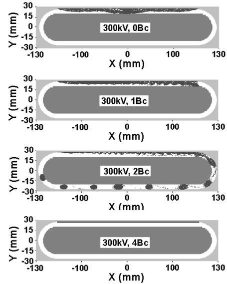
Figure 3: Snapshots of simulated electrons at 15ns.
