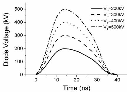
Figure 2: Waveforms of diode voltage for simulations.
