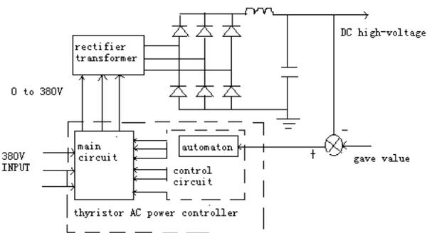
Figure 2: Control principle of thyristor AC power controller
