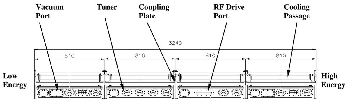
Figure 1. 3MeV, 350MHz, cw KOMAC/KTF Drawing.
