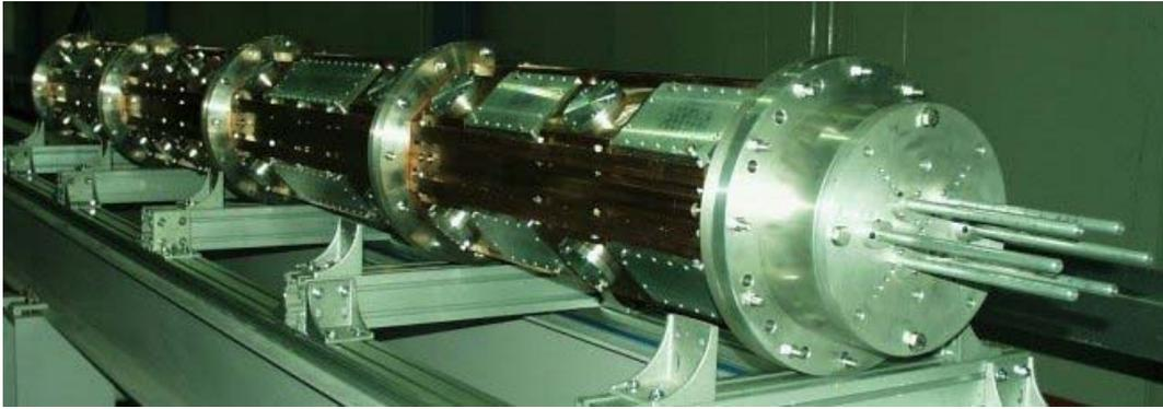
Figure 2. Fabricated RFQ cavity.
