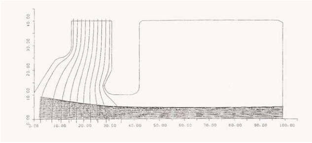
Figure 1 Computer plot of the gun optics at 160 kV showing equal-potential surfaces and the beam-focusing pattern. Shaded area denotes the electron beam. The emission current is assumed to be 12A.
