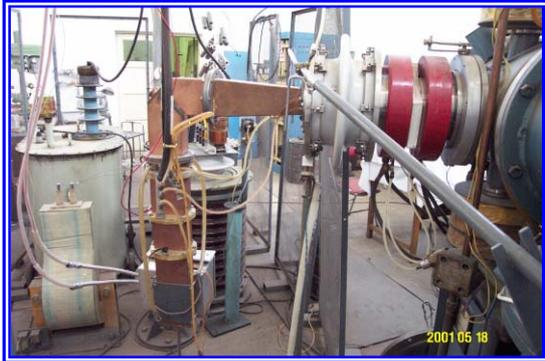
Fig 1: The ECR proton source in CIAE
