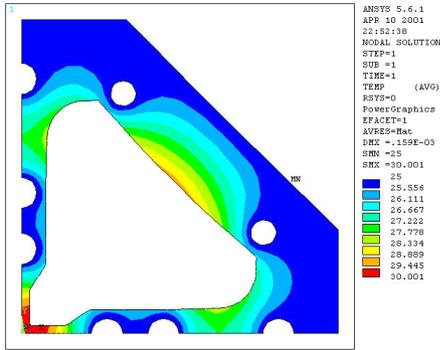
Fig. 5(a): Thermal and structure analysis for five cooling pipes
