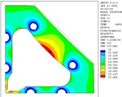
Fig. 5(b): Thermal and structure analysis for four cooling pipes
