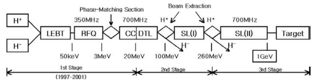
Figure 1: Schematic Layout of the KOMAC Linac
