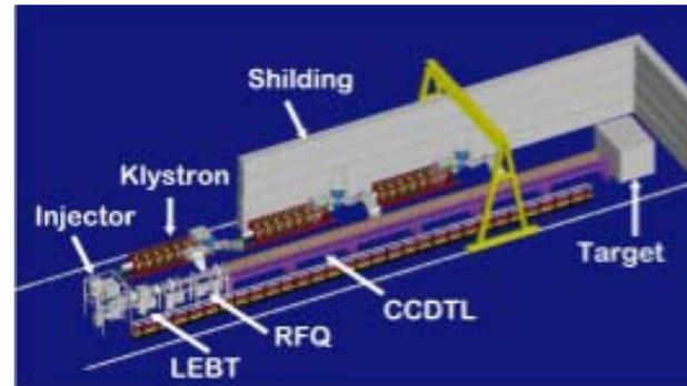
Figure 2: Plan of KTF 20MeV Accelerator
