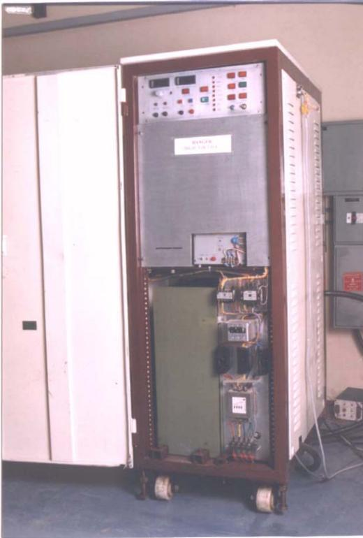
Figure 2: See From left Magnetron pulse modulator
