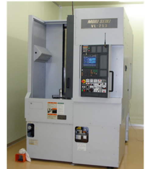
CNC vertical lathe (Moriseiki, Japan)
