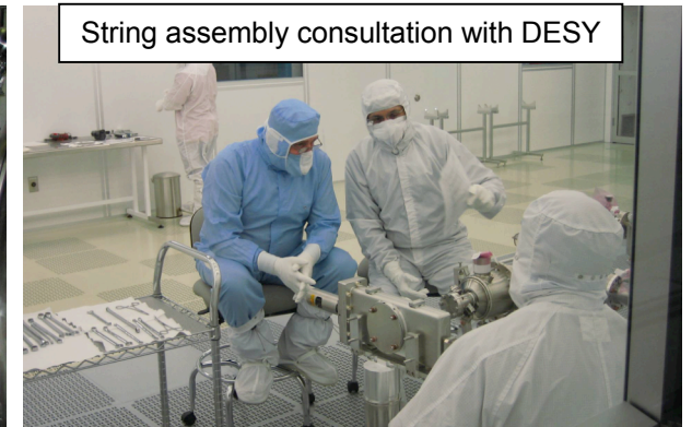
Preparing for mounting to cold mass
