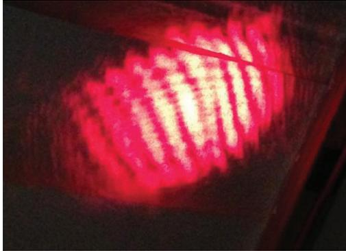
Figure 1: An interferogram of a ZnTe crystal with a physical defect. The curvy fringes are indicative of inhomogeneity of index of refraction through the material.
