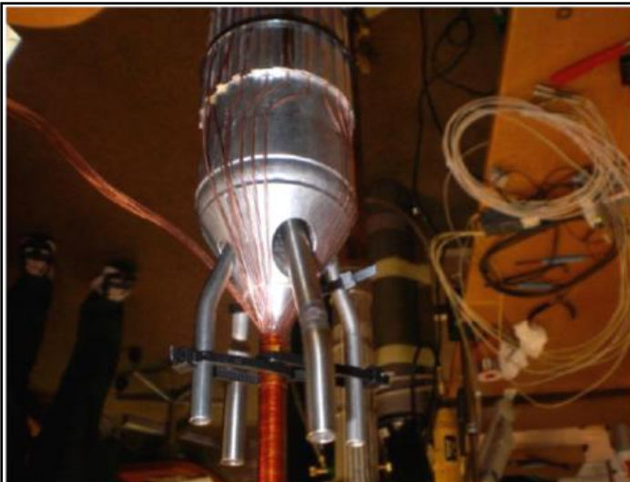
S.c. strands at the cold terminal connected to the HTS parts
