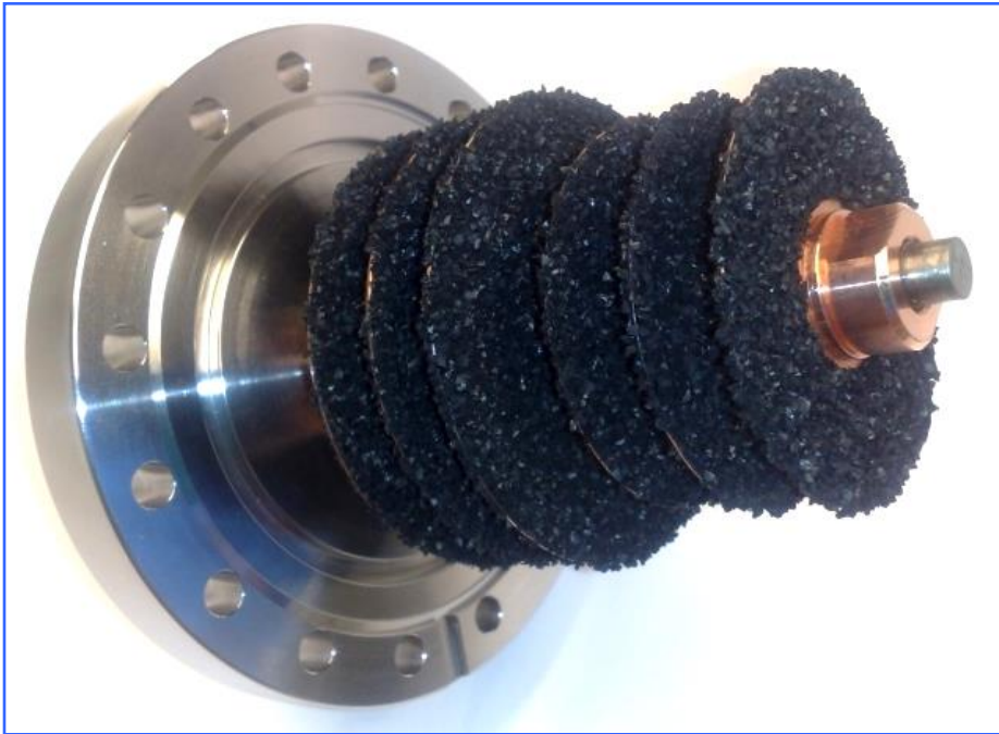
Adsorption pump produced at KIT, Karlsruhe
