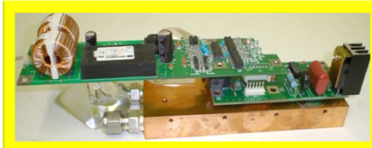
1 st Gen.: 0.7 kV Si-MOSFET board
