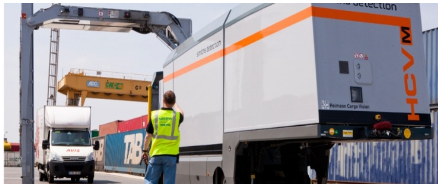
High Energy X-ray Mobile Screening System. Image Credited to Smith's Detection Systems. [f14]
