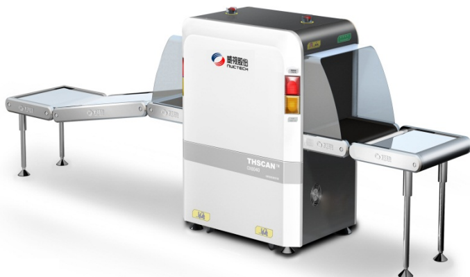
CX6040BI X-ray inspection system. Image Credited to Nuctech Company Limited [f9]
