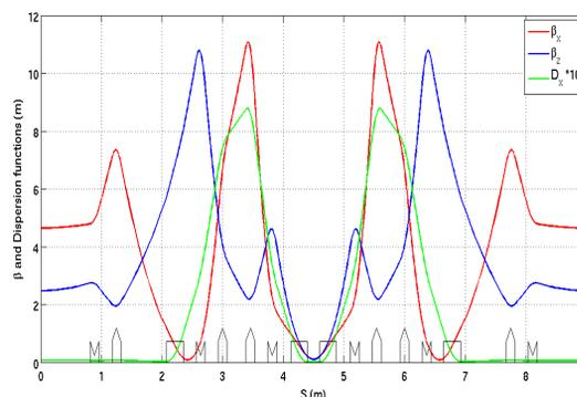
Figure 1: New optical functions for the ThomX ring.
