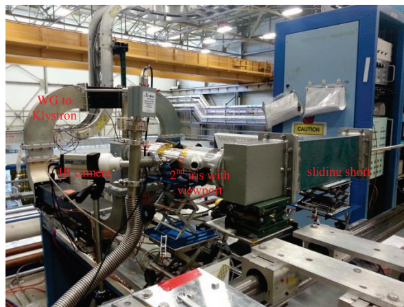
Figure 7: High power standing wave test setup; the traveling wave test used a water load to replace the sliding short in this figure.
