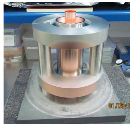
Figure 2: Outer conductor braze setup with the molly keeper ring.
