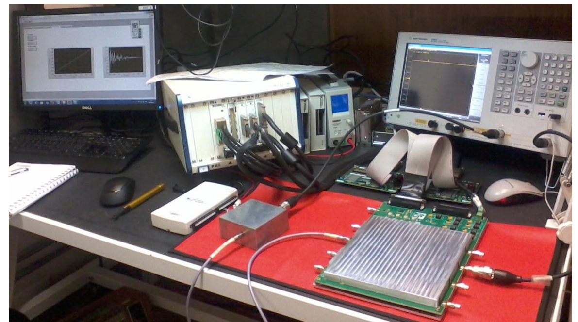
Nonlinearity bench test. Better results obtained with the RFFE and the “linearity box” in a temperature chamber.
