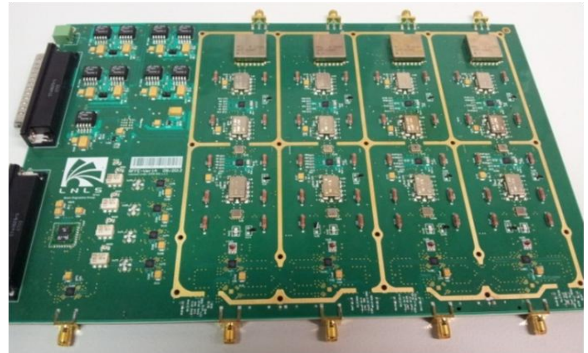
RFFE board. Ten layers of the Rogers RO4350 RF substrate.
