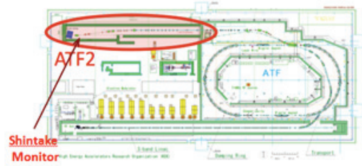
Figure 1: Location of Shintake Monitor in the ATF(2) beamline [3,7].
