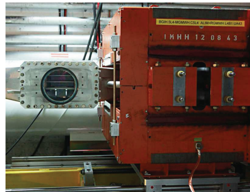
Figure 1: Up: a schematics of LHC BGI (from [1]). Bottom: a photo of the LHC BGI (flange with optical port) in the tunnel, with magnet displaced.
