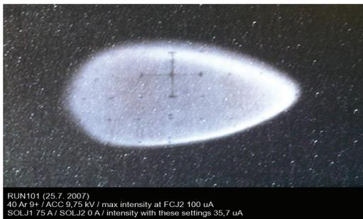
Figure 8: Asymmetric Ar<sup>9+</sup> beam after the dipole magnet.
