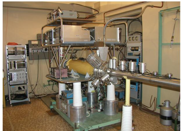
Figure 2: Electron String Ion Source Krion-2.
