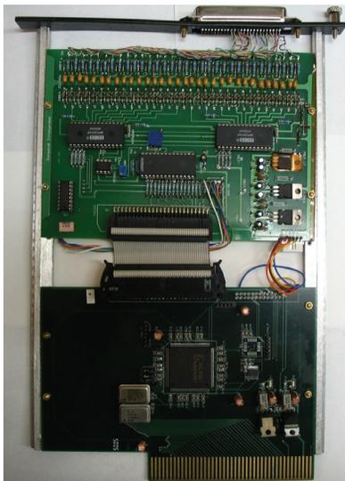
Figure 3: FPGA based CAMAC ADC module.
