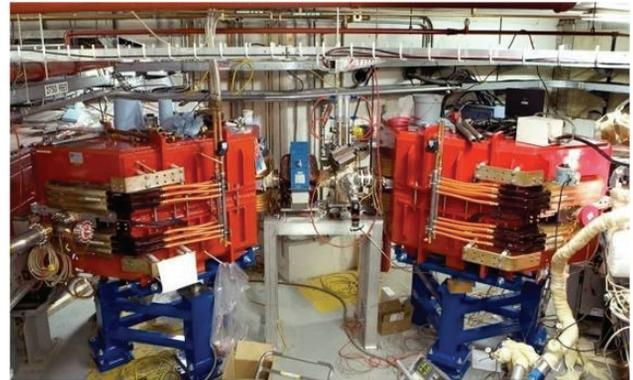
Figure 4: Dipoles installed in the Booster tunnel.
