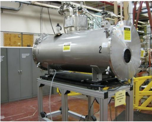
Figure 11: The 5 T, 2 m long EBIS solenoid at BNL.
