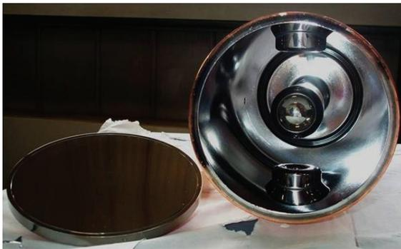
Figure 2: An upgraded medium  $\beta$  cavity with its tuning plate.
