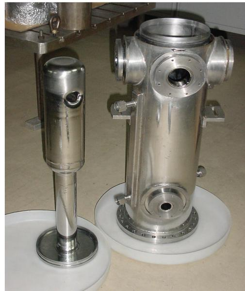
Figure 5: Central conductor and outer housing, along with its stainless steel jacket, of the resonator after the repair.
