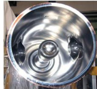
Figure 3: A newly designed medium  $\beta$  cavity.
