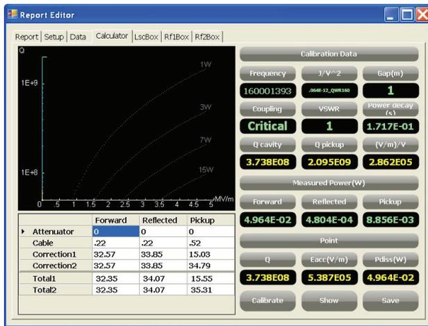
Figure 4. Options Window with RF Calculator panel.
