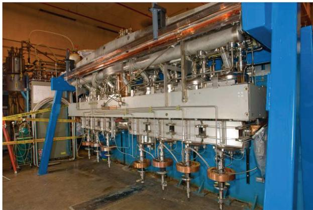
Figure 2: Cavity string suspended from the lid, with all cryogenic plumbing assembled and leak-checked, ready to drop into the box vacuum vessel.
