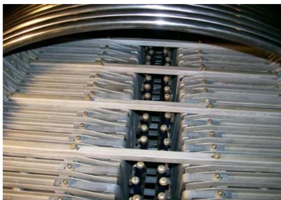
Figure 1: The new terminal voltage resistive divider installed between the column sections.
