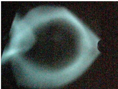
Figure 9: A hollow Ar<sup>8+</sup> ion beam after dipole.
