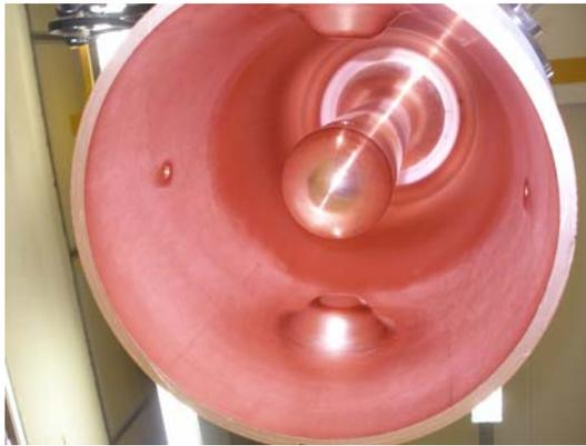
Figure 7: Cavity copper substrate towards final machining steps.
