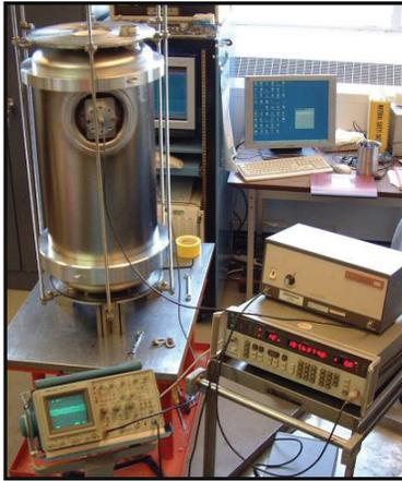
Figure 2: Parts clamped in *birdcage* for a frequency measurement.
