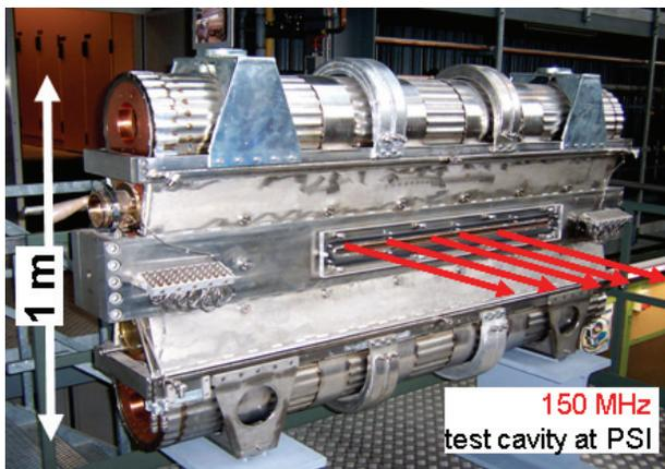
Figure 4: 150 MHz test cavity (single gap). A 92 MHz cavity is approx 1.5 times higher.
