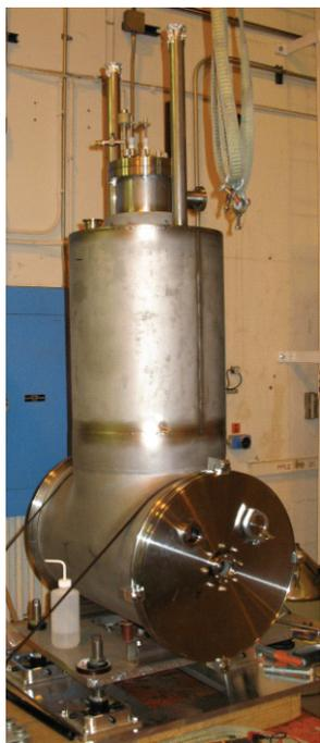
Figure 7: New solenoid in an individual cryostat.
