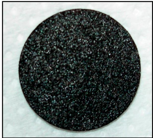
Figure 2: The first UCx pellet for the SPES project.
