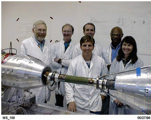
Figure 3: IR double-walled Be collision chamber with nearby water cooling and permanent magnet dipoles.
