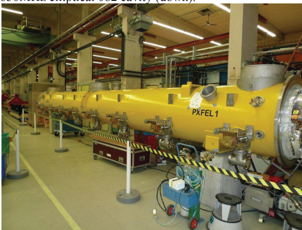
Figure 11: 12 meters long cryomodule for Euro-XFEL .
