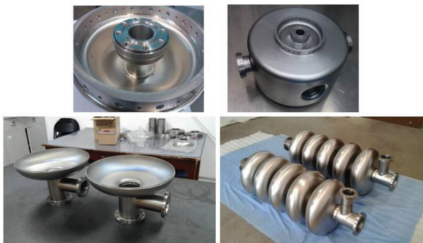
Figure 10: Superconducting spoke021 cavity (up) and 650MHz elliptical 082 cavity (down).
