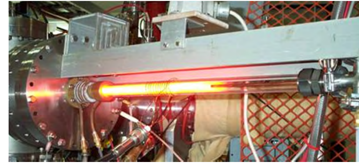
Hollow Cathode Ion Source based on design used on Saclay EBIS.
