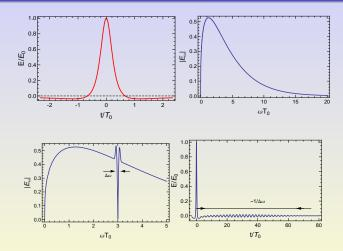
Sending radiation pulse through a thin crystal can remove a small part of the spectrum.
