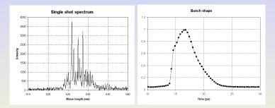
Measured fluctuating spectrum of synchrotron radiation at APS and inferred bunch shape, (V. Sajaev, EPAC2000). Fluctuations also occur in SASE FEL, however they are more complicated, especially in the saturation. See invited talk by M. Yurkov at FEL 2010. Fluctuations of a SASE FEL can be used for measuring the FEL pulse length<sub>42/55</sub>
