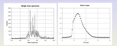
Measured fluctuating spectrum of synchrotron radiation at APS and inferred bunch shape, (V. Sajaev, EPAC2000).
