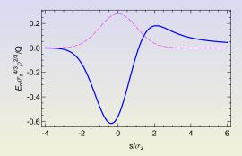
The head is accelerated and the tail slows down  $\rightarrow$  they move along different trajectories in the dipole  $\rightarrow$  transverse emittance growth.
