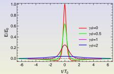
As  $\psi$  increases, the pulses become wider and smaller  $\to$  radiation is limited to small angles,  $\Delta \psi \sim 1/\gamma$ .
