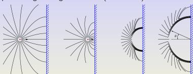
After the charge hits the metal it disappears, and an expanding spherical wave annihilates the electromagnetic field moving with the charge. Radiation field is localized in a thin spherical shell. For a relativistic particle,  $\gamma\gg 1$ , it is concentrated at small angles,  $\theta\sim 1/\gamma$ .
