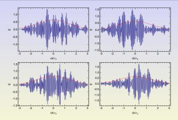
One can see about 10 coherent regions in the field pattern [ $10 \approx c/\sigma_z \Delta \omega$ ]. Measuring fluctuational properties of the radiation one can infer the beam profile.
