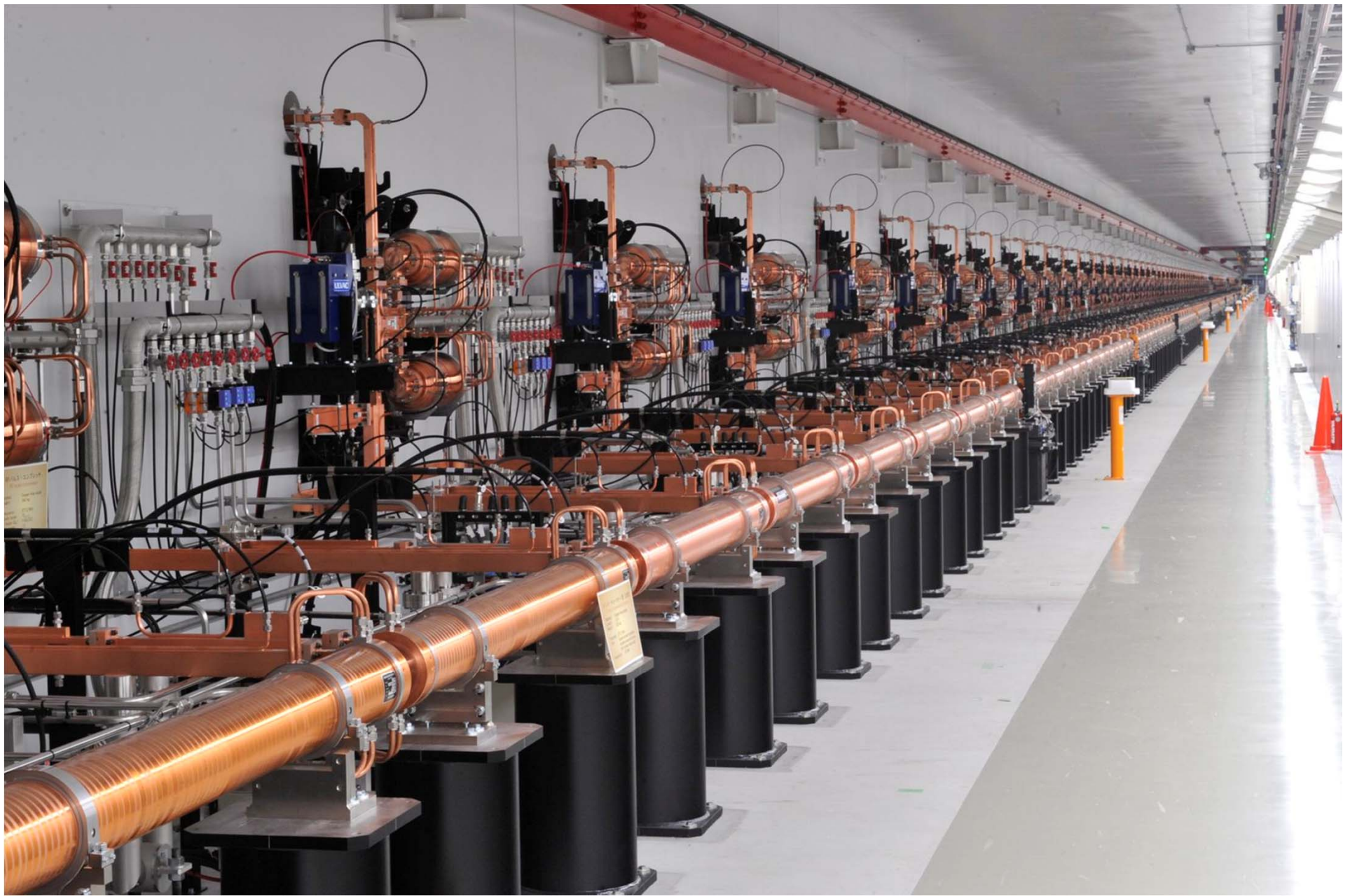
400m, 8 GeV Accelerator with C-band running at 35 MV/m
