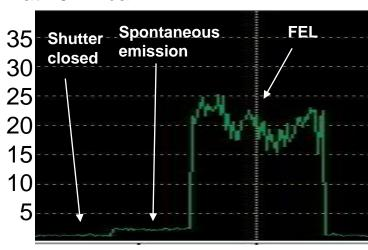
About 8\*10<sup>8</sup> photons per pulse (at **43nm**), equivalent to **6nJ**.
