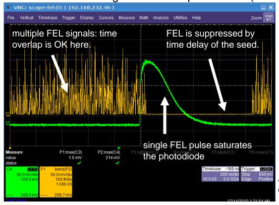
Shot-to-shot signal [a.u.] from atomic photo-ionization of Nitrogen at 10<sup>-5</sup> mbar.
