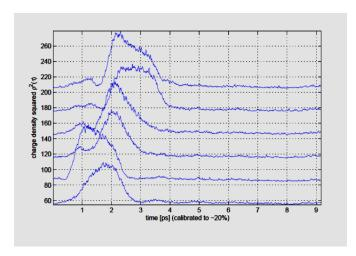
Electro-optic bunch profile measurement (ZnTe crystal probed by Ti Sapphire laser)
