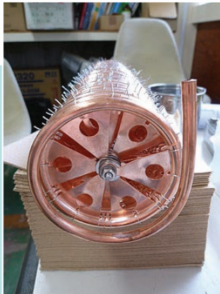
Heat Exchanger Fin made by punching press
