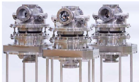
Three 2-cell cavities with 5 HOM couplers
