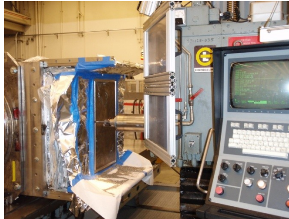
Cutting the cryostat open
