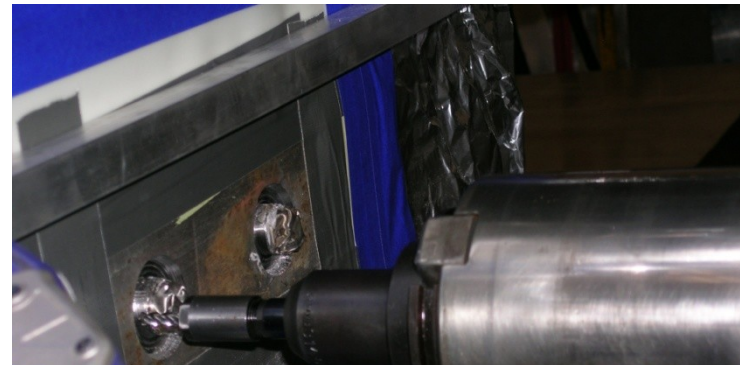
Replace fill tubes 2/2010 without damaging the SC wires
